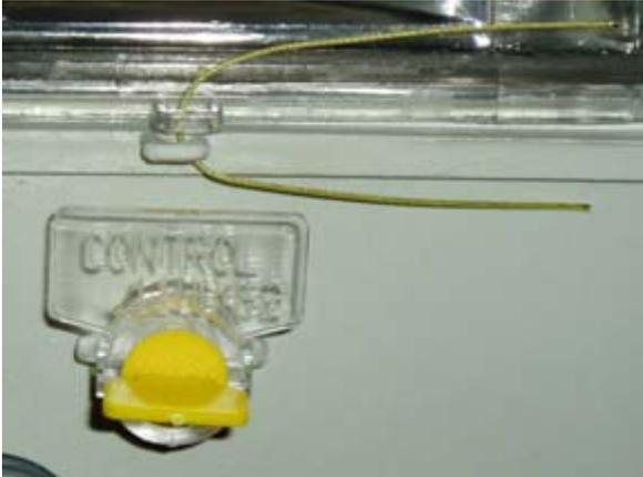
**2.** Thread free wire ends through holes in seal body, closing the seal to 30 mm to the object being sealed.
