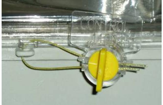
**3.** Rotate drum flag clockwise till making maximum pull-up of sealing wire.
