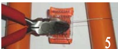
5. Nip free overhung ends of flexible-body.
