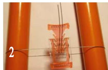
2,3,4. Holding the seal at the minimum distance from the object of sealing, push in the bending cue into the bottom of fir-tree cue until bumping.
