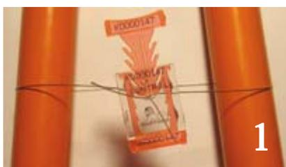
1. Thread free ends of flexible-body through holes in seal body, moving the seal closer to the minimum distance to the object being sealed.
