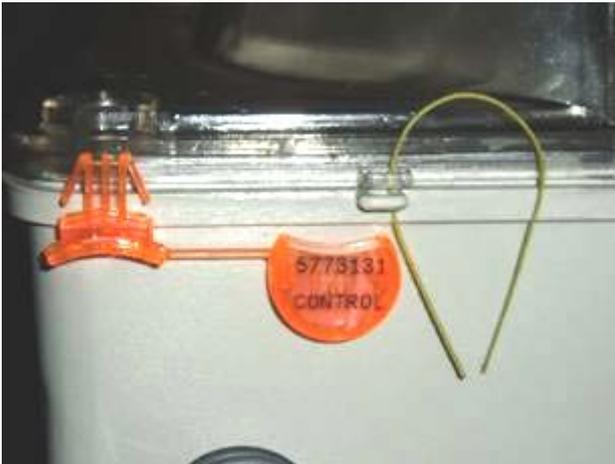
**2.** Thread free wire ends through holes in seal body.
