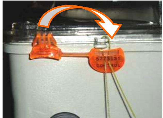
Holding wire in the drawn state, move the seal closer to the minimum distance to the object being sealed.
