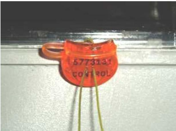
**4.** Nip ends of wire, hung over the seal body limits, by side-cutting pliers.
